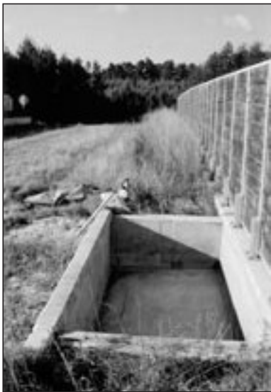
Fig 6. The same fragment of the bridge surface presented in Fig. 5. In order to precisely weigh the soil and the lower layer of fine filtering stones, the contents of container 1 were taken out and weighed
